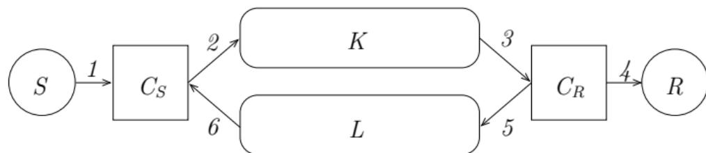
The protocol entities are a sender  $S$ , a receiver  $R$ , a forward channel  $K$ , and a backward channel  $L$ .
